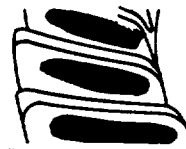
Figure 8-3. Proper pinion-to-differential ring gear tooth contact pattern.
